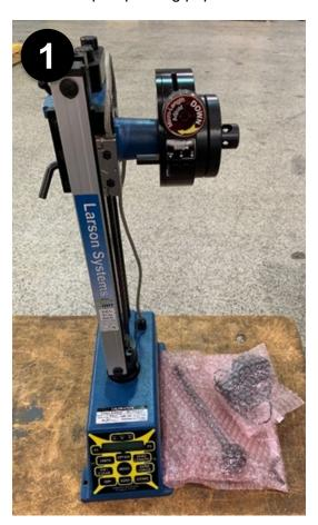
2. Adjust the upper assembly so the distance between the blue castings is 5.25 inches and make sure the upper and lower platforms are not touching one another. Tighten the three Quick Release Handles / clamps on the upper assembly so it does not move up and down the support rods.
