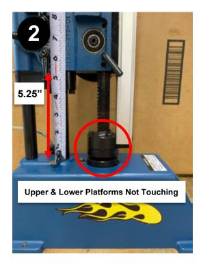
Engage the micro length adjust (if you have one) and tighten the gear rack lock knob. If you have quick release handles, face them forward.
