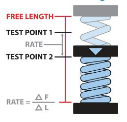
Test two points to get a free length calculation in one spring deflection.
