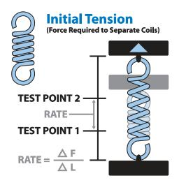
Test two points to get an initial tension calculation in one spring deflection.
