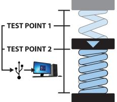
Test ир two preselected force length points in one spring deflection without stopping.
