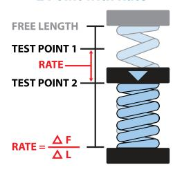
Test two points to get a spring rate calculation in one spring deflection.
