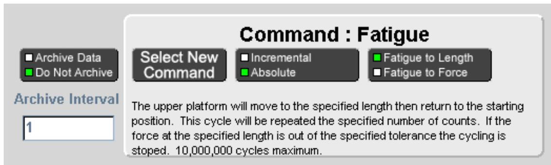
The fatigue test can be programmed to stop in the event of part fatigue or breakage. By entering a nominal force or length and a tolerance value, the part is checked when the platform stops at the target position. If the part does not test within the specified tolerance, the Fatigue test will stop.
