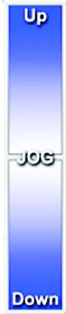
The **Jog Bar**, located on the left side of the display in Manual Mode, controls the movement of the upper platform. Touch and hold anywhere on the Jog Bar to engage it. The platform moves faster when the darker portion of the Jog Bar is touched and slower when the lighter portion is touched. It stops when the Jog Bar is released.
