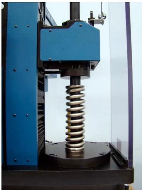
The STAR offers thru-rod testing capabilities up to 2 inches in diameter, so you can test long, flexible or buckling springs without worrying about safety. Improved stroke and range enhance extension up to 78 inches! Limit switches at the top and bottom act as a failsafe for the software stops and the load cell's physical stops. They are redundant protection to safeguard over-travel and component damage.
