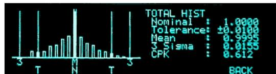
A histogram of all parts produced since the count was reset to zero. Includes statistics and 3-sigma, mean, nominal and tolerance markers.
