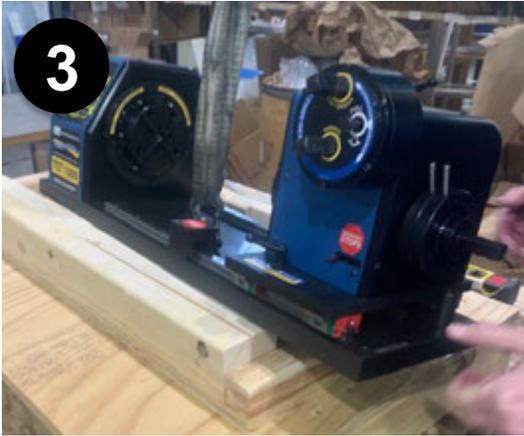
4. Lock the inverted carriage stop and the rotation lock in place.
