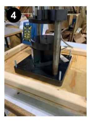
5. Add a rubber washer (to protect finish), metal washer, and a locking nut to the carriage bolts and tighten.
