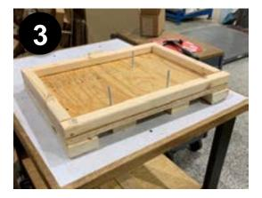
4. Lower the tester onto the carriage bolts in the bottom of the crate.
