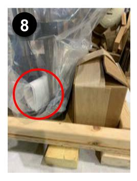
9. Cover the tester with a plastic bag and tape or shrink wrap in place. This helps to keep it clean. Include some desiccant packets to absorb moisture during transit.
