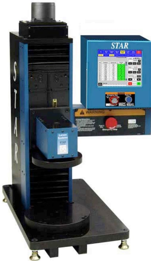
The STAR offers three standard drive units with an 11" stroke or a 1,000-lb unit with a 25" stroke. Nine interchangeable load cells are available for this model--use one machine to test from 0.5 grams up to 3,000 pounds.
