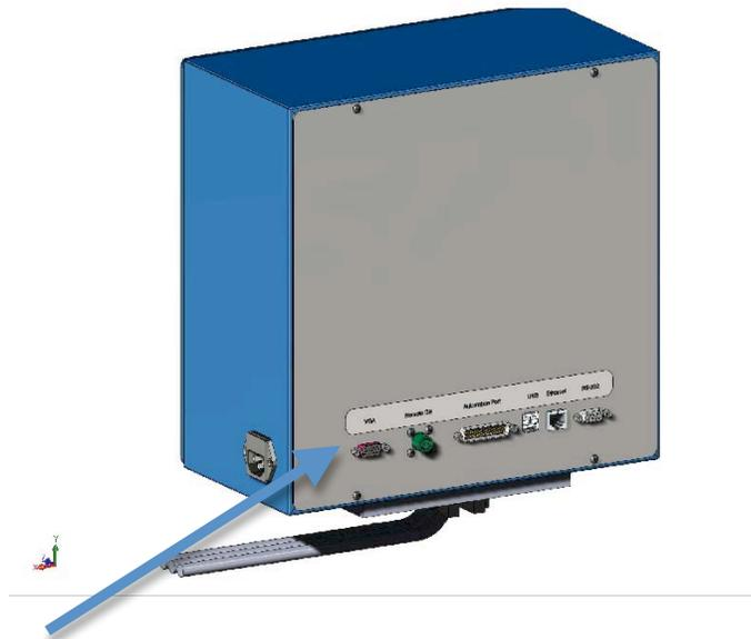
The FLASH head now includes an optional VGA connection to allow you to attach a video monitor to the tester and view operations from a remote location. A USB port allows connection to a monitor and keyboard for remote operation.
