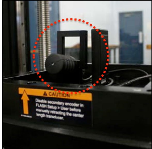
Clamp shown in the extended position.
