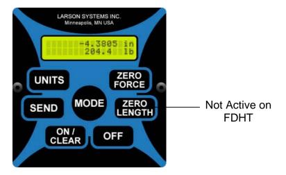
**[UNITS]** Choose unit of measurement – lb, N, oz, or kg for force and in or mm for length. **[MODE]** Select the test mode that applies. The test modes available are: Manual (or Tracking) and Peak (if enabled). A mode for Shunt calibration verification is included. **[ZERO FORCE]** Zero out the current force reading displayed.
