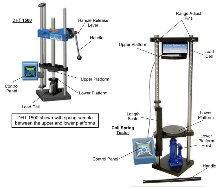
The DHT 1500 and CST shown are the heavy-duty versions of force spring testers produced by Larson Systems and are designed with a two-column structure to accommodate larger force capacities and sample parts. The FDHT 1500 (not shown) is similarly equipped to the DHT 1500. Some of the structural differences are:
