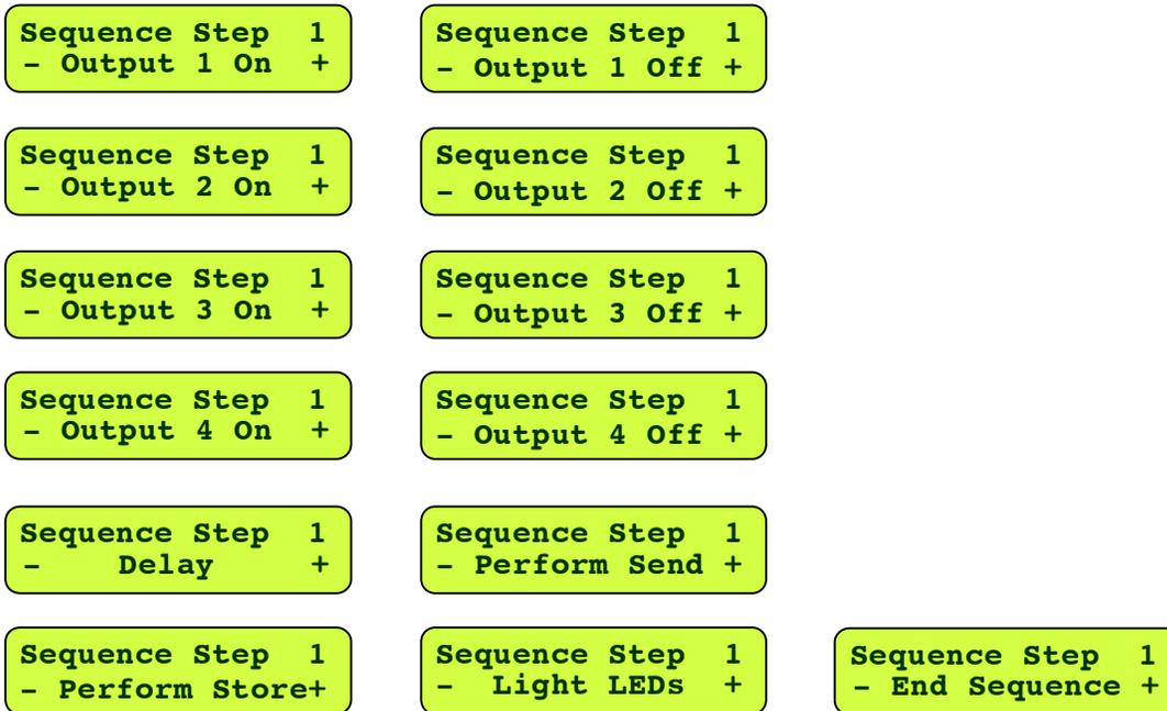
A single iteration is usually made up of multiple Sequence Steps. For each sequence step, choose one of the available selections shown above. To make a selection scroll to the selection desired and press [OPTION]. Once a selection is made, the display advances to the next step:
